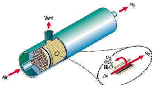
Membrane separator cross section
